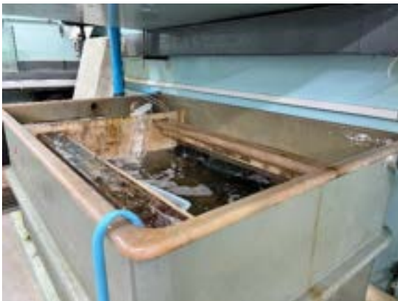
Figure 24: Simple trickle biofiltration systems that are used for the experimental systems
