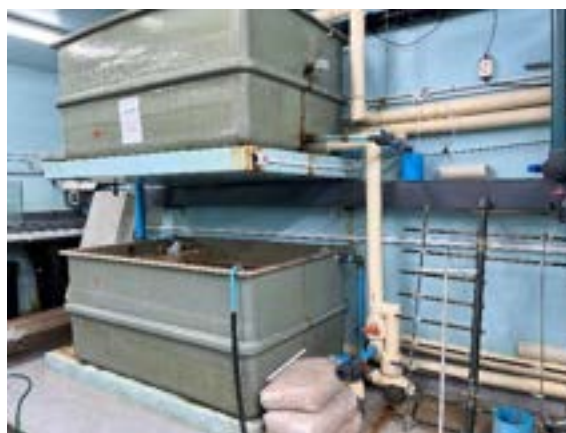
Figure 24: Simple trickle biofiltration systems that are used for the experimental systems
